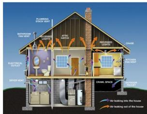
such as blower doors, which measure the extent of leaks in the building envelope, and infrared cameras, which reveal hard-to-detect areas of air infiltration and missing insulation
